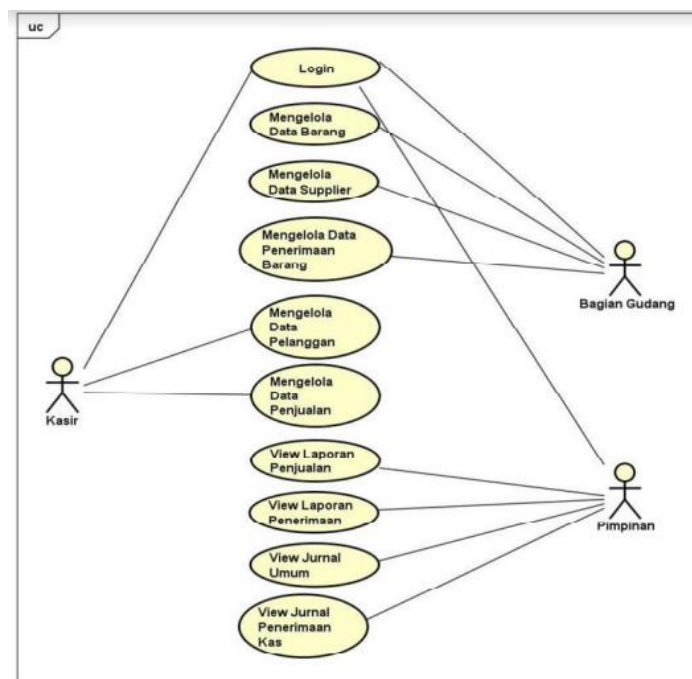
Gambar 1. Use Case Diagram.
